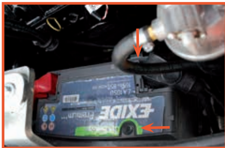
Maintenance free battery with charge indicator. Self-bleeding electric pump to bleed air from the injection system.
