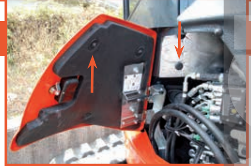
Linings fixed with press studs (not just glued in place).
