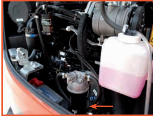
Sensor that indicates by means of a light if there is water in the filter.
