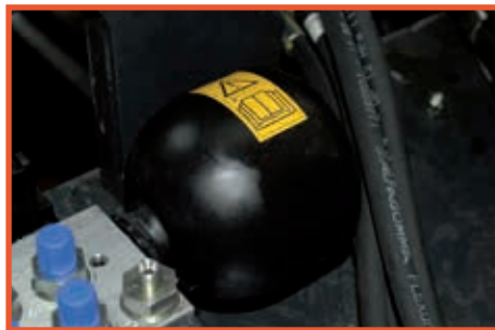
Accumulator to allow pressure discharge from auxiliary pipelines with the engine off.
