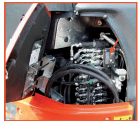
Fuel pump with automatic cut-off if over-full or no diesel in drum.
