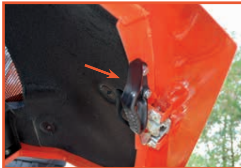
Practical internal handle for lowering the cover.
