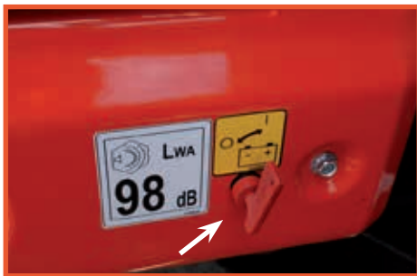
Battery isolator key to prevent battery running down during long downtimes.
