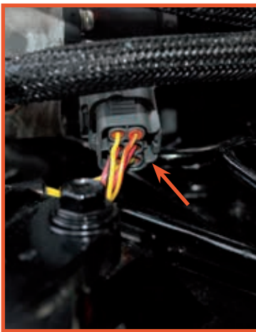
IP67 watertight electrical connections.
