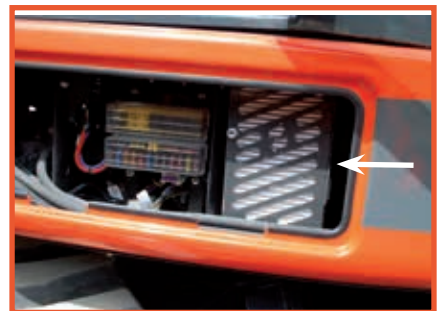
Easily accessible main air filter.
