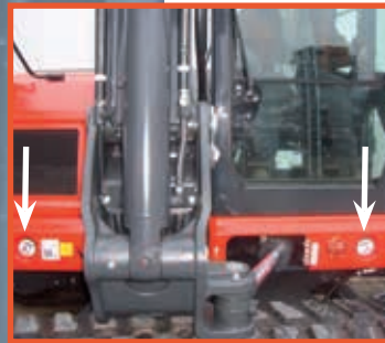
2 lights for the work area on the turret and 1 protected light under the boom.
